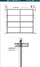
The Urban opening solution is a counterweight balanced, vertical lift bi-folding system constructed from structural steel and is suitable for all application types. By eliminating the need for overhead structure, architects and customers will have more clear opening to create amazing views and access.
